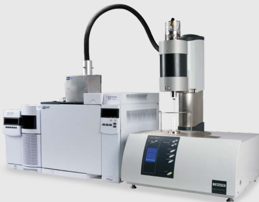
Standard STA 449 F1 Jupiter ® coupled with the GC-MS via the heated transfer line
